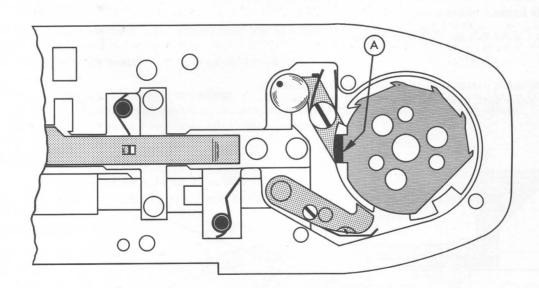
b) Replace bushing and gear assembly and balance of components with exception of setting rack.
