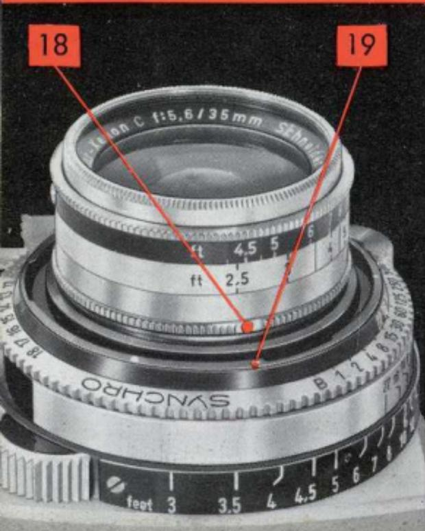
The front component of the RETINA lens is interchangeable. To remove the standard lens, rotate it anti-clockwise as far as it will go, and lift out of the shutter. We recommend the use of the special lens container designed for the standard lens for easy changing and convenient storage.
