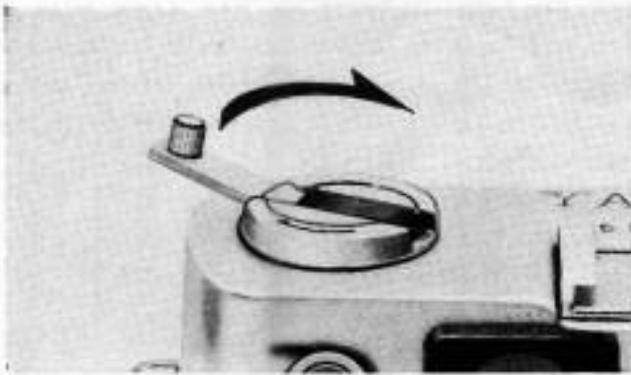
Flip up the film rewind crank handle to the horizontal position and wind in the direction of the arrow. Toward the end of the film you will feel a slight resistance, but continue turning the rewind crank until the film pulls away from the slot on the Take-up Spool.
