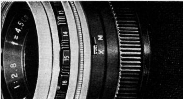
The synchro-selector lever must be moved to the "X" position when using the self-timer.
