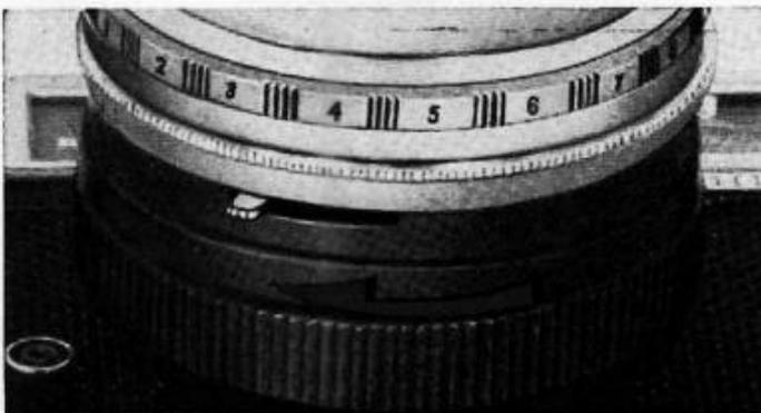
Set the speed and move the self-timer lever to the direction shown by the arrow. The self-timer runs about 8 seconds before the shutter snaps.
