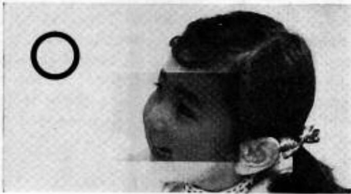
The left photo shows that the super-imposed image and actual one overlaps and forms a clear image, i. e., the camera is in true focus.
