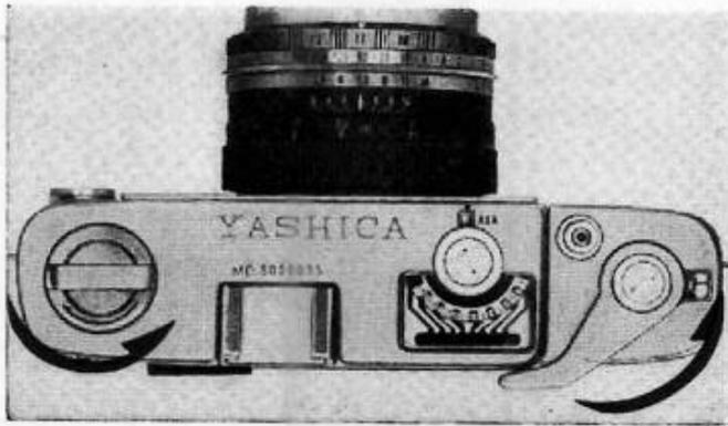
When cocking the advance lever, be sure to observe the rewinding knob turning in the same direction simultaneously. If it does not, the film leader has slipped from the take-up spool. You must then open the back cover and rethread film.
