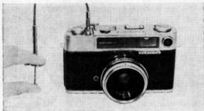
A standard cable release can be fitted to your Yashica. Screw the Cable Release into the socket provided on the Shutter Release Button.
