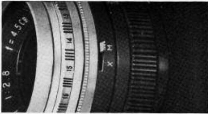
Move the MX Synchro Selector Lever to the "M" position, when using M-type bulbs.
