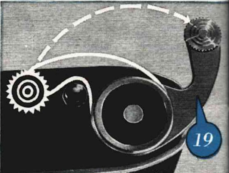
ment. This at the same time tensions the shutter and — when the camera is loaded with a film — winds on the film by one frame and advances the film counter (see page 13).
